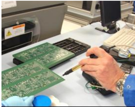
Figure 25: Measuring PC conductor with high impedance Contact Voltmeter
