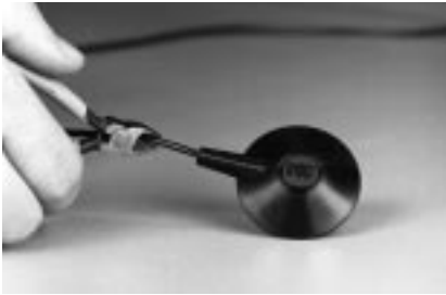
Fig. 6 - Cutting off table mat ground snap.
