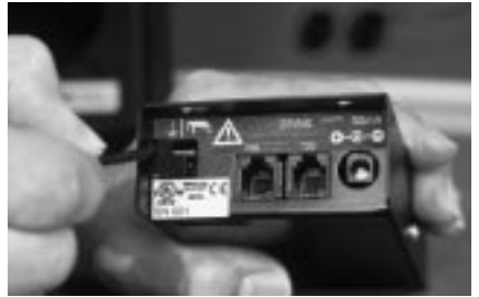
Fig. 8 - Inserting two-wire connector into rear of Model 724.
