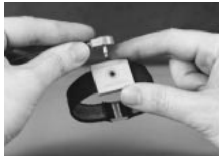
Fig. 13 - Connecting ground cord to wrist band.
