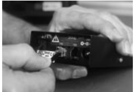
Fig. 9 - Inserting 732 plug into rear of Model 724.
