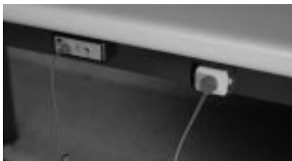
Fig. 15 - Attach cord to Model 3057 standby jack.
