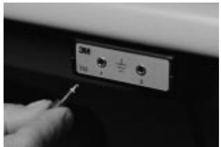
Fig. 14 - Connecting wrist snap ground cord to Model 732.
